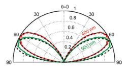
Directional emission at  $\lambda$ =500 from a Au nanoparticle optical Yagi-Uda antenna excited at the left-outmost particle, with emission observed towards the right.
