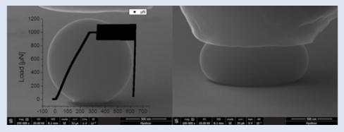
Silica particle compression with 1 mN DC, 100 µN @ 10 Hz AC load. Particles shown exhibit viscoplastic creep under load.
