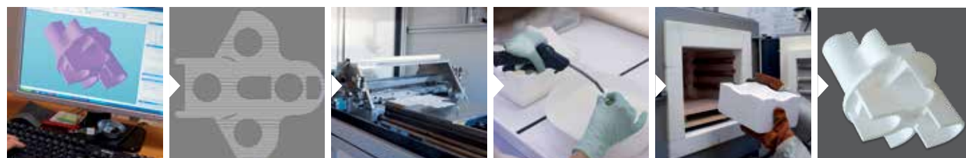
Creation by CAD Slicing of the parts before printing 3D printing Cleaning Debinding and sintering Finishing
